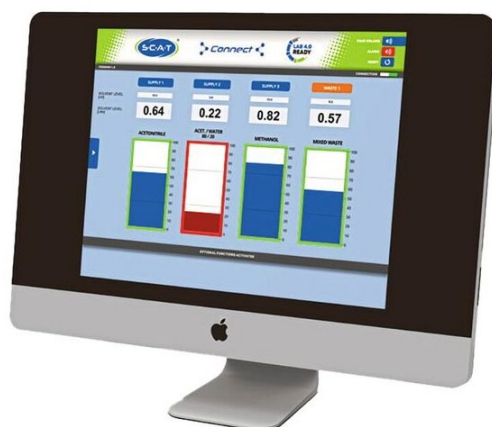
Fig. 3: With the app for SCAT-Connect, users in the laboratory always have an eye on the fill levels of their solvents.
